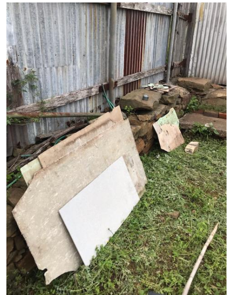
Legacy Asbestos at Residential Property
